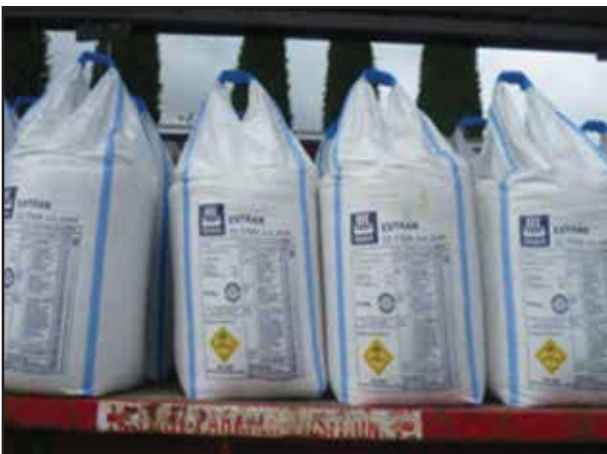
Not secured in a curtainsider – unacceptable.
